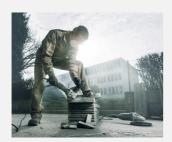
In crafts and landscaping, professionals using the WE 19-180 Quick RT can cut 60 millimetre thick patio and paving slabs as well as roofing tiles with one cut. Therefore, the WE 19-180 Quick RT has the same cutting depth as a large 230 millimetre angle grinder, however, is only half as heavy.
