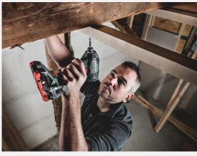
With its powerful brushless motor, the impact driver drives screws in soft wood up to a diameter of 8 and a length of 300 millimeters. **Photo: Metabo**
