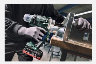
Practical feature: Integrated retainer mouthpiece holds the rivet in any position; this means it can't fall out while you're working, no matter what position the device is held in.
