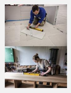
Using the LOCK function, you can use the TECH 700 DA as a bevel gauge: easily transfer the measured angles onto a part.
