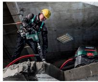
make even difficult demolition and drilling applications easy. The vibrations are dampened in two ways by means of a decoupled handle and an impactabsorbing counter-oscillating mass.
