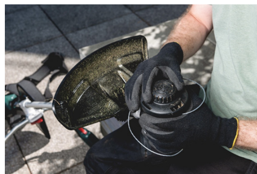
Quickly and without tools: Users change the line in the Metabo brush cutters FSB 36-18 LTX BL 40 and FSD 36-18 LTX BL 40 without opening or having to remove the spool.
