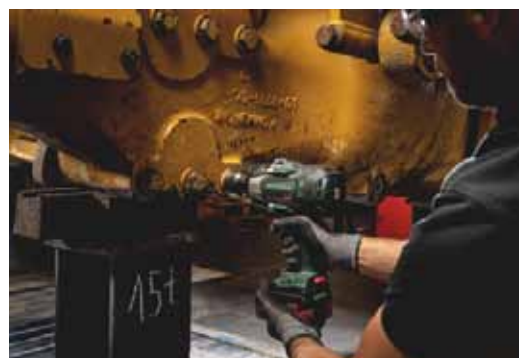
Delivers on its promises: The cordless impact wrench handles screws up to M33 and is suited for the most diverse jobs on construction vehicles. Photo: Metabo
