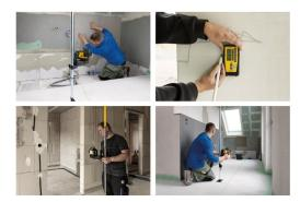
Thanks to GreenBeam technology, it's possible to work directly on the sharp green lines of the LAX 600 G multiline laser from STABILA at distances of up to 40 metres. Photos: Stabila
