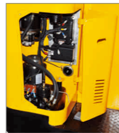
Vertically mounted drive motor with CANbus technology reduces wiring complexity and increase reliability.
