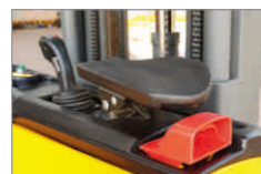
Finger-tip joystick and adjustable arm support
