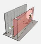
MANUAL ALIGNMENT: using the remote control (A), the LAR 350 laser (B) is moved accurately to the REC 300 Digital target point (C).
