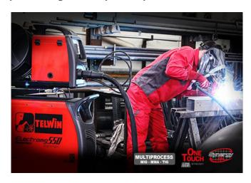
This is Electromig 550 Synergic, a powerful multi-process MIG-MAG inverter welding machine (MIG-MAG / FLUX / BRAZING; MMA and TIG DC-Lift) suitable for a wide range of applications from the industry to metal processing. Excellent striking and control of the arc, together with the constant monitoring of the main welding parameters directly on the wide LCD display, make it possible to increase the quality of work (thus reducing the time required to remove welding spatters).
