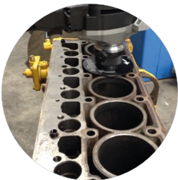
Versatile deburring and chamfering of contours, radii and countersink holes, 30° weld seam and visual edge preparation etc.
