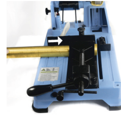
4. The next workpiece is brought into the position to be sawed.
