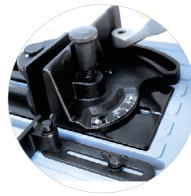
MITER CUTS CAN BE ADJUSTED WITHOUT TOOLS 90-75-60-45°
