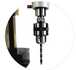
Twist drilling with CM3-adapter
