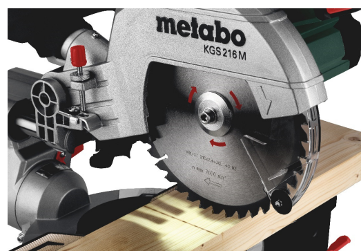
The Precision Cut Line projects a precise shadow line on the material and thus replaces the single line laser. The shadow always shows the tooth width of the saw blade and thus the precise cutting line. Even when the saw blade is changed, no adjustment is needed and the Precision Cut Line can be used on both sides. Photo: Metabo
