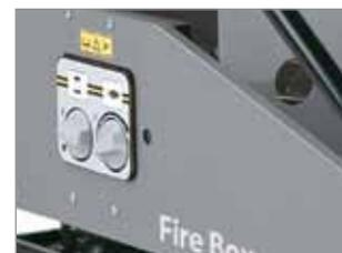
ELECTRIC CONTROL PANEL WITH ON-OFF SWITCH AND THERMOSTAT
